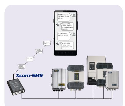
The **Xcom-SMS** is a cost effective add-on to your system easy to install and a plug-and play solution. It provides a secured access to your installation by the simplest way: sending or receiving SMS to your remote power system.
